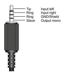
Note: For connection to Mic or Headset inputs: adjust headroom in Toolbox between "0dBint=-22dBFS=-14dBu" and "0dBint=-30dBFS=-22dBu" for low output level to avoid distortions caused by input overload.
